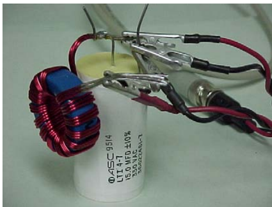
Figure 3. Single-Stage Filter Construction and Test Leads.
