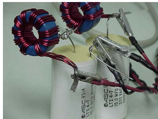
Figure 4. Two-Stage Filter Construction and Test Leads.
